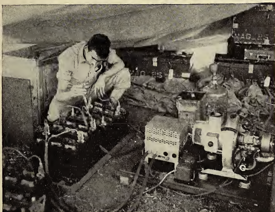
Airplane batteries are recharged in this "hangar." Extra care is necessary because spare parts are virtually nonexistent.
